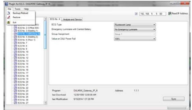
If you need to exchange a device, you can load the backed-up data onto a new device via Restore. Backup – Restore gives you the opportunity of a simple device exchange without the time-consuming post-installation. We therefore strongly recommend that you create a back-up and save the data after completing the parameter settings.
