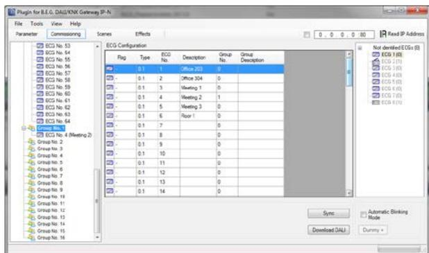
Once an ECG has been dragged into the ECG configuration table, it disappears from the list of non-identified ECGs. The 'PLAN' flag in the configuration table shows that the ECG has been assigned to the planned element. If an ECG has been wrongly assigned, it can be moved back to the list of non-identified devices using the same drag& drop mechanism.
