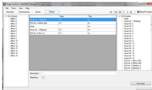
Use the fields 'Value' and 'Time' to set the final value to which you would like to dim a group or ECG as well as the dimming time for each effect step. If you are setting a delay, the entry in the 'Time' column shows the length of the delay. Use the descriptions field underneath the effect steps to enter a user-friendly name for each effect. Tick the 'Repeating' box if you would like the selected effect to run continuously.
