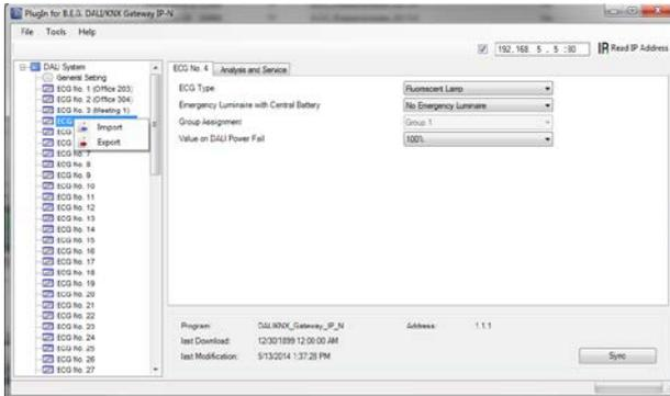
If you would like another ECG to have the same parameter properties, simply select the ECG and import the exported file into the new ECG. The file serves as a template for other ECGs. You can also create templates at group level or for 'General Properties'. Creating templates for all ECG and group types and using this template library makes the configuration, especially in large installations, significantly easier.
