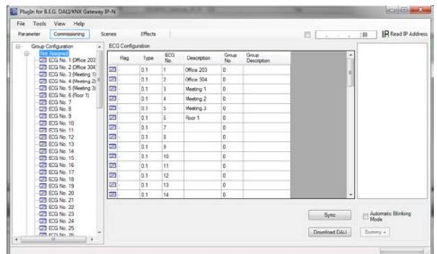
The structure of the commissioning page is as follows: The group configuration is displayed on the left-hand side in a tree structure. The area in the middle shows the ECG configuration and names in a table format. On the right hand side is a list of all devices found in the system, which have not yet been identified. During the planning
