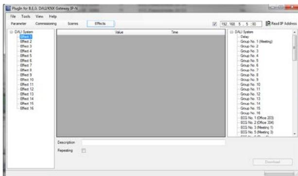
Go to the Effects page and select the required effect from the directory on the left-hand side. Move the groups and individual ECGs which are needed for this effect from the directory on the right-hand side into the field in the middle using drag-and-drop. The order of the entries corresponds to the order of the individual effect steps. You can also use drag-and-drop to move the delay times into the table and to change the order of items within the list.
