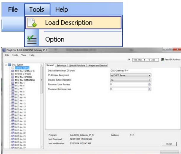
As loading the names via KNX can take quite some time, you should use the Ethernet connection for this process. Before starting the process, please make sure you set the right IP address and tick the check-box in front of the address.
