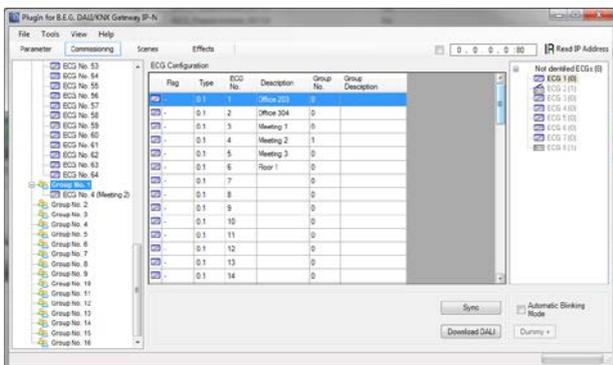
You can now identify the devices by switching the corresponding lamp on or off. If you select an ECG and press the right mouse button, a context menu appears from which you can select the required function.
