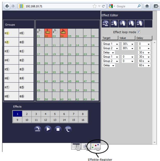
To program an effect, select it first from the effect block at the bottom of the page. (If the effect has been previously programmed, the corresponding effect steps are displayed in the Effect Editor on the right hand side of the page.)
