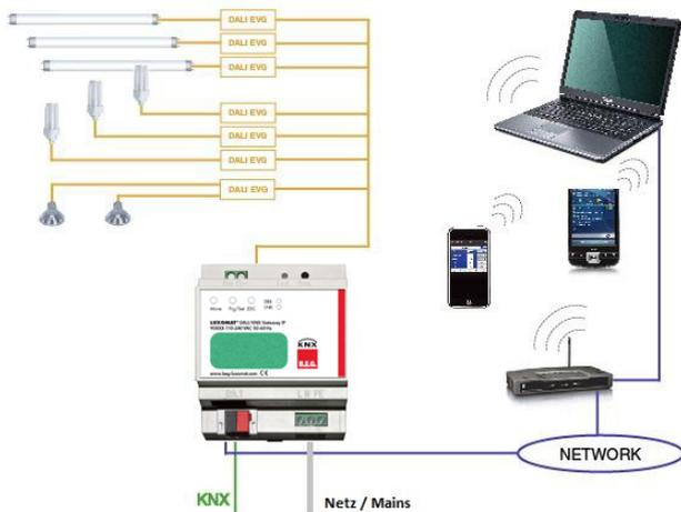
Use a standard patch cable to connect the device to a switch, hub or router of the IP network. You can also use a WLAN access point as network coupler. This means you can commission the DALI via a portable note book, tablet PC or mobile phone.
