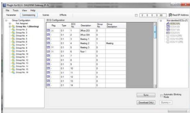
Use this button to add dummy ECGs to the list of non-identified ECGs.
