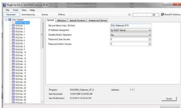
Start the synchronisation via the sync button in the bottom right-hand corner of the main window. Depending on the size of the installation the synchronisation may take a few seconds. A bar at the bottom of the page shows how far the synchronisation has progressed. When the synchronisation is complete, only the objects and parameters of those ECGs that are physically connected to the device are shown.
